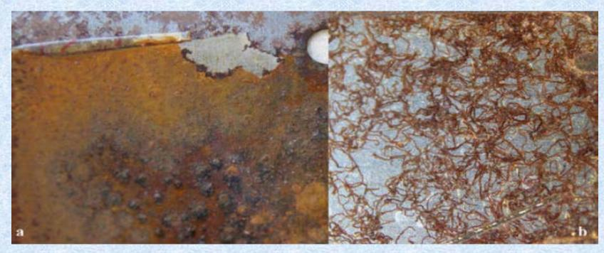
Fig. 3. Corrosion of steel substrates after 1 week of immersion in 5 wt.% NaCl (aq) solution, coated with a PBDMA based coating (a) and filiform corrosion underneath a PSMA based coating (b).
