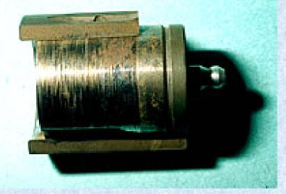
Friction-wear at an axle-cylinder contact point.
