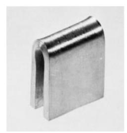
FIG. 10 A Bent Copper-Copper Sulfate-Sulfuric Acid Test Specimen
